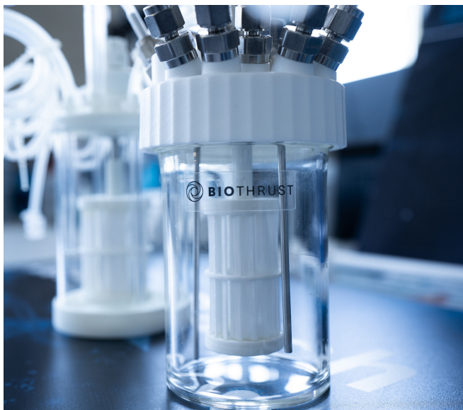
Figure 1: In the foreground, the ComfyCell reusable bioreactor vessel. In the background, the single-use version of the ComfyCell, referred to as the ComfyCell SU300.
